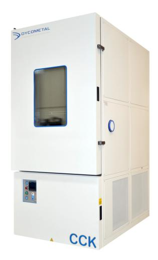
Climatic tests on specimens can reproduce the climatic conditions of temperature and humidity, which will be subjected during its lifetime. This will provide for their behavior in environmental conditions of use, transport and storage, preventing defective product hits the market.
