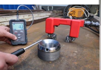
Gaussmeter (magnetometer) NOVOTEST MF-1 is designed for rapid non-destructive testing and allows:
